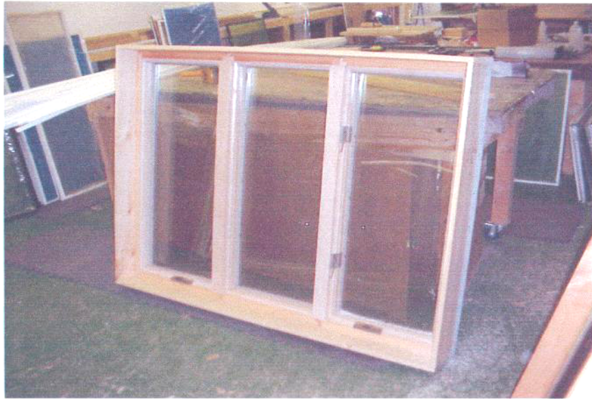
Three Casement Windows Mullered Together Before Installation
