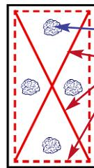
Note: 2 cans of Professional Wide Web Spray Adhesive and 4 tubes of PSA-29 Acoustical Panel Adhesive are needed for 16 - 2' x 4' panels.
