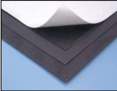
**VB-2** provides a clean flexible solution for vibration damping sheet metal panels. They effectively eliminate noise emanating from resonant structures and surfaces. Outstanding damping characteristics are achieved by overlapping filler platelets which are oriented during production. Such materials achieve a high degree of damping over a broad temperature and frequency range.
