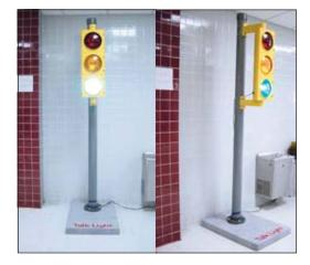
The Talk Light stand provides the flexibility to move the light to different locations within the room or out of the room as needed. The pole is 8' tall and is secured to a base that was designed for the traffic light.
