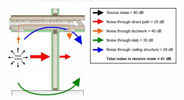
This diagram illustrates some simple flanking noise paths. The red arrow is direct sound - what you would measure in a lab to arrive at an STC rating, etc. - the green and blue paths are some simple "flanking paths". Often, these paths are more important than the direct, yellow, path at many frequencies.
