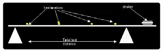
Nonetheless, this simple test illustrates, conservatively, the performance of the Green Glue in this regard. This diagram illustrates the basic test set-up.
