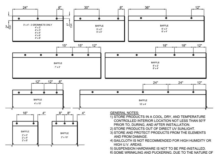
7) BAFFLES ARE CONSTRUCTED FROM FIBERGLASS WITH A SOFT AND FLEXIABLE CORE. GROMMET LOCATIONS MAY VARY.
