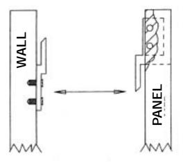
· For all ceilings apply a small amount of adhesive on both parts of the brackets. Slide brackets together.
