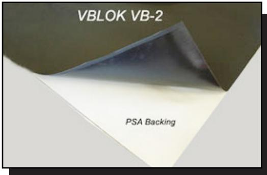
VB-2 is a high-performance, lightweight, vibration damping sheet that has been engineered to convert vibration energy into low level heat through viscous friction. VB-2 vinyl damping materials feature a silica-mica and ceramic mineral load. This product offers significantly higher damping performance than asphalt based materials. VB-2 is highly moldable and features an aggressive acrylic adhesive which allows for 100% adhesion to a vibrating structure.
