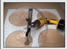
Cut holes in drywall and ceiling tile quicker, cleaner, and more affordably when installing audio speakers.
