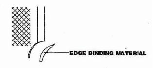
2) FOLD EDGE BINDING MATERIAL OVER EDGES, EQUAL AMOUNTS ON FRONT AND BACK
