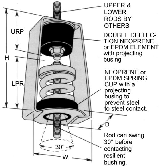
**Type 30N Spring Hangers** feature a lower rod that can swing up to 30° for ease in installation to compensate for misalignment. Spring and neoprene element in conjunction remove high and low frequency noise.
