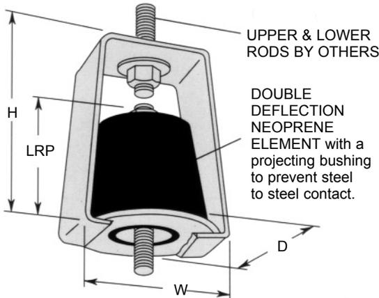
HD Neoprene Hangers offer the same increase static deflection and vibration control as ND mounts but in a sturdy steel hanger box.
