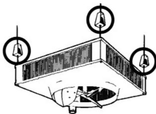
HD hangers perform the best when used on equipment located adjacent to stiff support walls and columns, and suspended from narrow rigid upper building spans.
