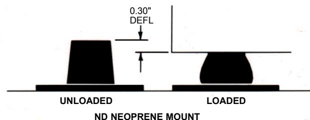
(unless stacked), so they act mostly as noise breaks. They interrupt hard surface-to-surface contact and reduce high frequency vibration. 2) Neoprene mounts and hangers deflect more and are the first step in true vibration control. 3) Spring isolators have the greatest deflection for maximum vibration reduction.
